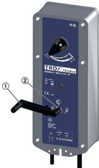
Fig. 47: Functional test (without power supply)
